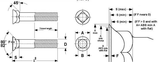
Length of plow bolt is measured from the top of the head to the extreme end of the bolt.
